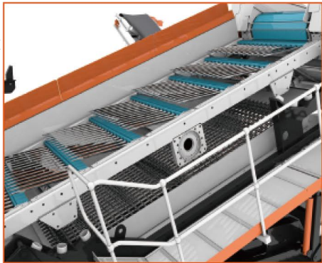
Screen box structure
